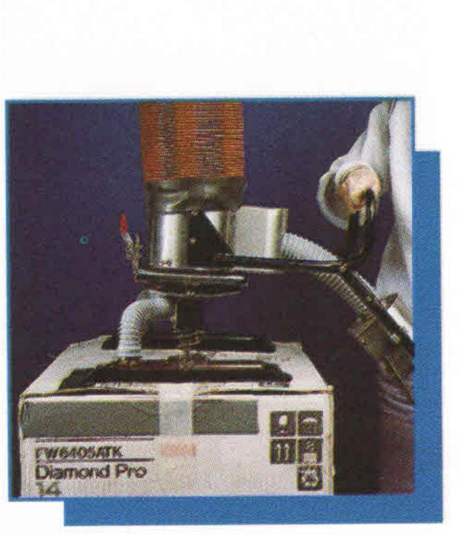
Two adjustable circular pads (24" yoke; 7.75" diameter pads) Gasket: 10651 Application examples: Large TV screens, double pails.
